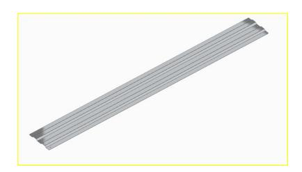
Weight of the gravel loading: Evenly filled grooves, about 16kg per plate; about 10kg per plate per aditional cm of fill
