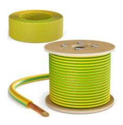
Halogen free according to EN 60754 1/2-1-2 - Radial water blocking cable - Flame retardant according to UNE-EN 60332-1 and IEC 60332-1 - Conductor category class 5 - Nominal voltage [V] H07V-K: 450/750 V - Isolation resistance: > 20 M $\Omega$  x km - Fire behaviour: VDE 0482-332-1-2/IEC 60332-1
